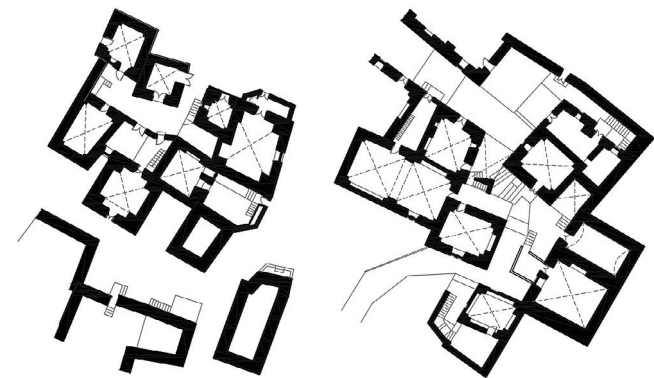
Рис. 7. Дома с внутренним двором – хошем (Mollenhauer Anne. Historical residential houses in As-Salt remarks on their shape and function. Annual of department of antiquities of Jordan. 1997. 234 p. )
